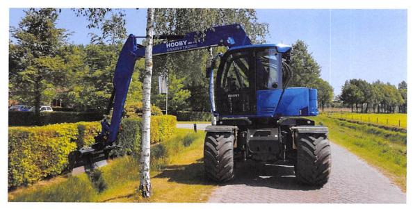
With the rotating boom it is possible to empty the bucket in line with the driving direction.
