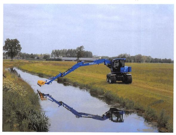
Cutting narrow shallow ditches is no problem with the additional extension boom.
