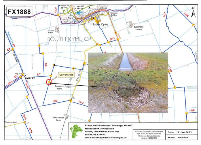
This culvert has partially collapsed, the blockage removed by the Board.
